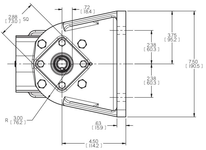
ROCESS UNLESS OTHERWISE SPECIFIED ASME Y14.5M-1994. ASME Y14.5M-1994. COMMENTS: SUCTION STRAINER AND DISCHARGE RELIEF VALVE MUST BE PROVIDED. ALIGNMENT: UNITS ARE ACCURATELY ALIGNED AT THE FACTORY. ALIGNMENT SHOULD BE CHECKED BEFORE STARTING TO ENSURE THAT IT IS STILL WITHIN .005 (0.133 FIM. PRESTARTING: FLUSH SUCTION PIPING BEFORE CONNECTING PUMP. PRIME AND VENT PUMP. READ INSTRUCTION MANUAL FOR DETAILS BEFORE STARTING.
