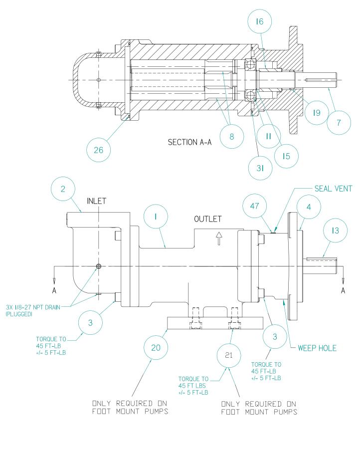
Fig 5 - Steel Pump Assembly
