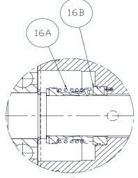
Elastomeric Bellows Mechanical Seal w/Spacer
