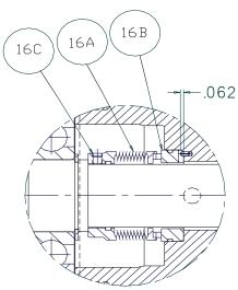
METAL BELLOWS MECHANICAL SEAL
