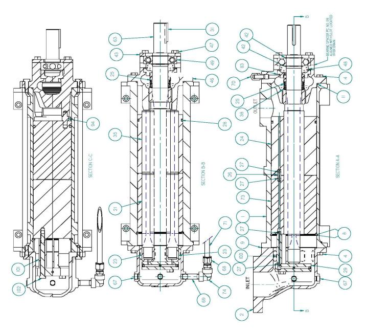
FIG. 9 - G6D-312 FOOT MOUNT PUMP ASSEMBLY
