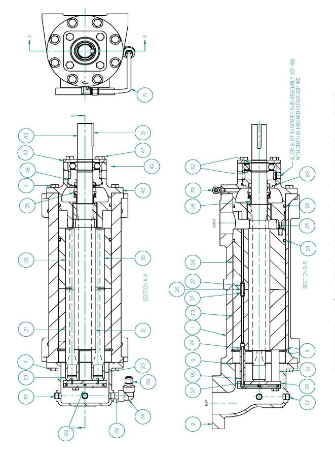
FIGURE 7 - G6D-275 FOOT MOUNT PUMP ASSEMBLY
