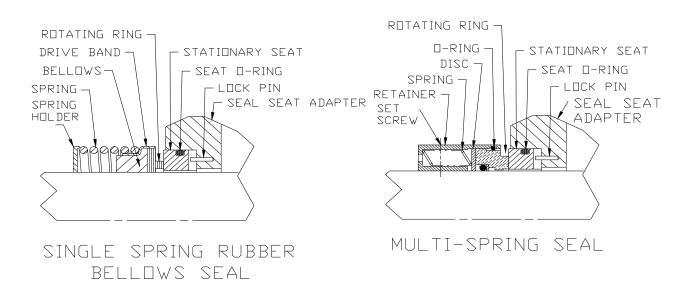
FIGURE 2 - Seal Drawing
