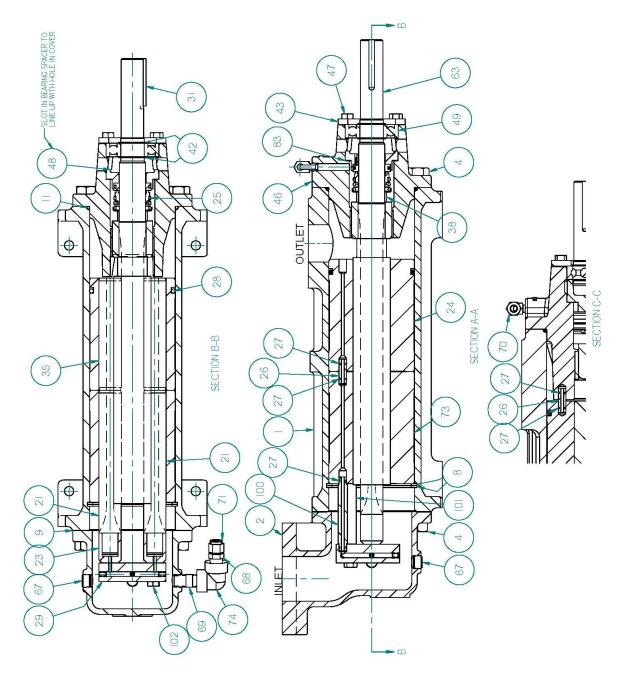
FIG 5 - G6D-218, 250 FOOT MOUNT PUMP ASSEMBLY
