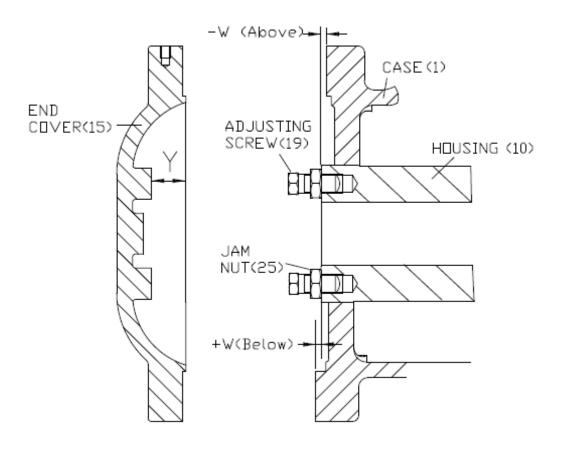
Figure 3 - Set Adjustment Screws, Outboard End
