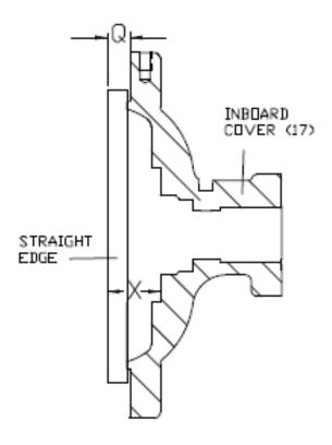
Figure 2 - Set Adjustment Screws, Inboard End
