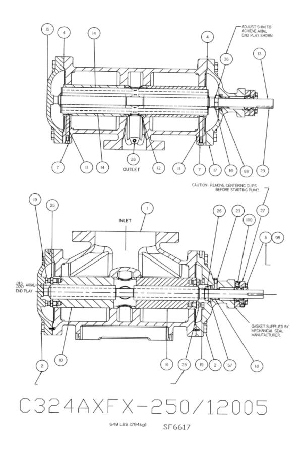
Figure 4 – Pump Assembly Drawing
