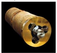
Incorporating a third idler rotor in the Imo design (one power rotor and three idler rotors) automatically creates a complex internal leakage path, providing a restricted interconnection among cavities. Pressure rise therefore is more constant and gradual. Bubble implosion is less abrupt
