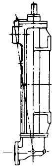
SCHEMATIC OF OIL RETURN LINE FROM SEAL CHAMBER FOR STD INLET POSITION
