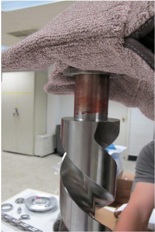
Slip the shoe onto the idler. Use arbor press to seat sleeve if necessary.
