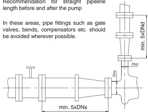
**ATTENTION** Shorter pipelines on the suction side are possible, but may lead to a deterioration of the hydraulic performance data. Shorter pipelines on the discharge side are possible, but may lead to increased noise development.
