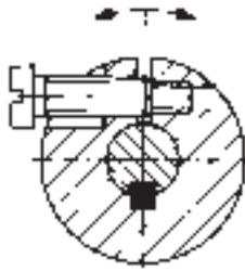
Tighten forcing screw with a screwdriver, but not using excessive force.
