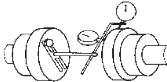
Figure 5.3: Alignment of the coupling with dial gauges
