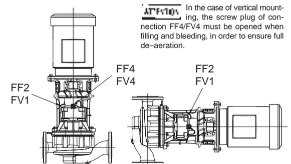
It may be necessary to twist the housing cover (161.01) in relation to the volute housing (102.01). The gasket (400.01) must not be damaged during this process. Replace if necessary.
