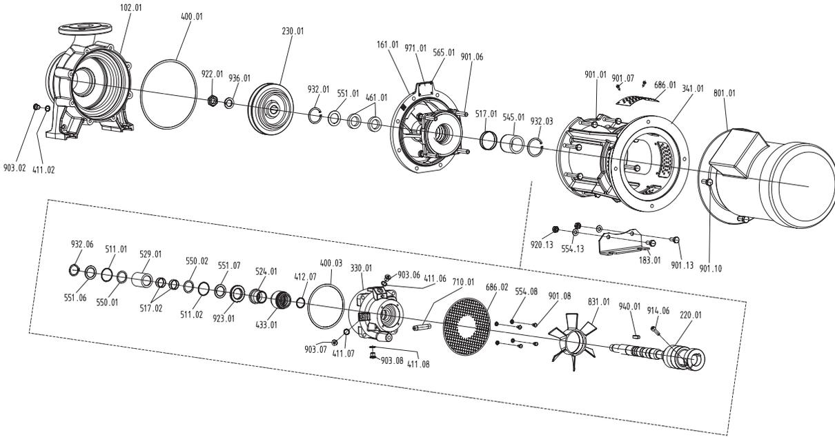
Design U3.3A–K1 (unbalanced mechanical seal with carbon-bearing)
