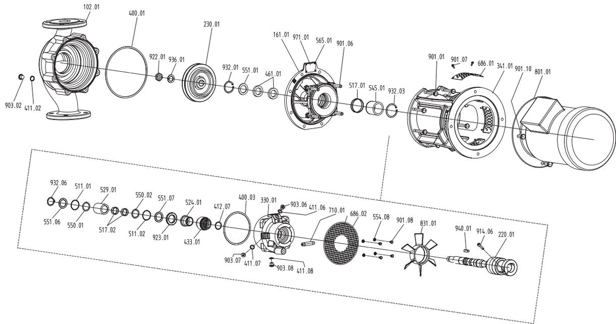
Design U3.3A–K1 (unbalanced mechanical seal with carbon-bearing)
