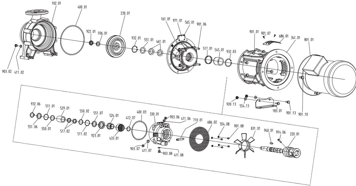
Design U3.3A–K1 (unbalanced mechanical seal with carbon-bearing)
