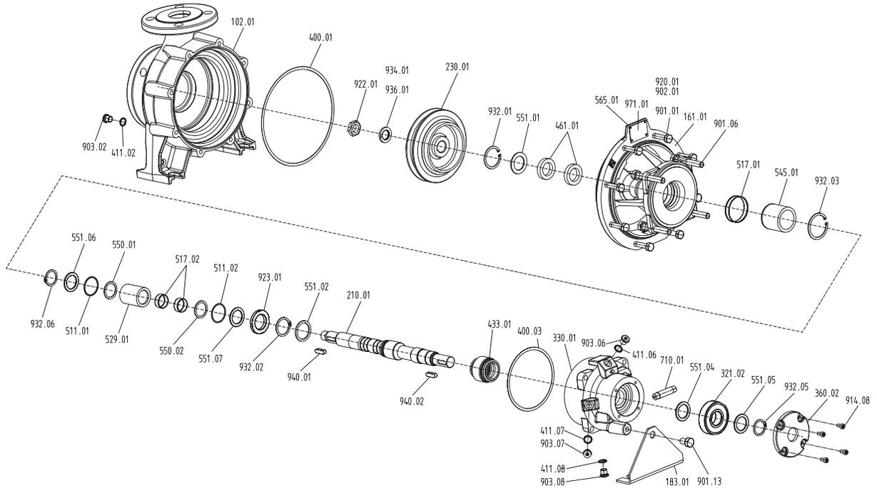
Design U3.3A-K1 (unbalanced mechanical seal with carbon-bearing)
