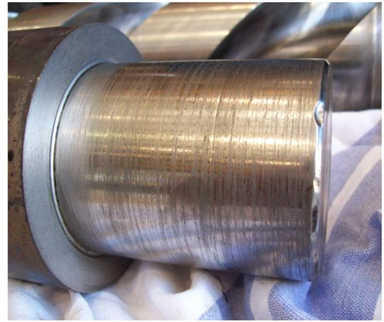
Idler cup and shoe normal wear in an application with high sand content. Bottom of cup (left) shows some damage where metal has been “picked out”- possibly cavitation.
