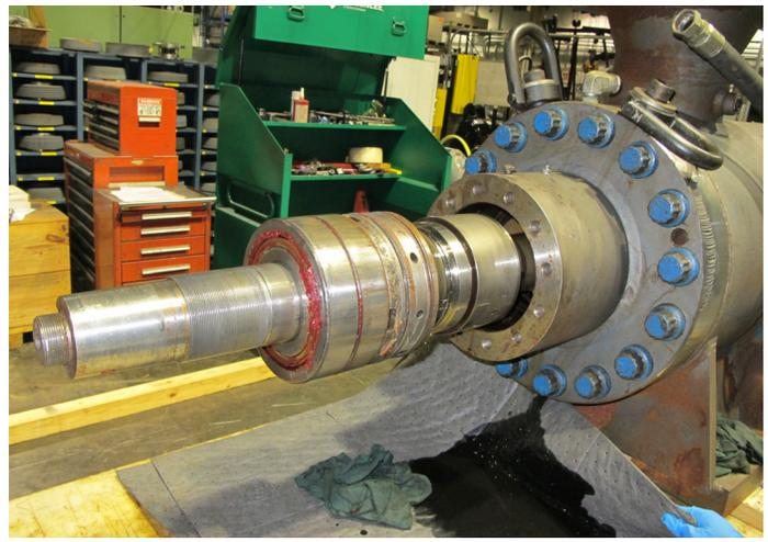
**LEFT** – Pressing power rotor out of inboard cover. If shaft is to be reused, ensure a blank is placed between power rotor removal strongback (S626MN) and outboard end of power rotor. **RIGHT** – Mechanical seal/bearing installation.
