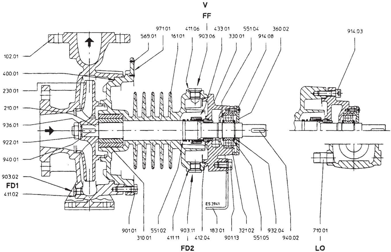
Shaft seal: Uncooled, balanced mechanical seal
