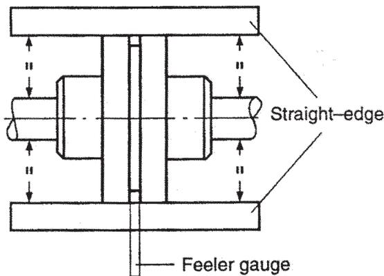
Fig. 4: Alignment of the coupling with straight-edge and feeler gauge
