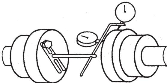
Fig. 5: Alignment of the coupling with dial gauges
