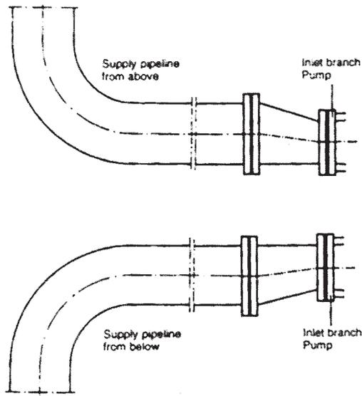
Fig. 6: Laying of pipelines
