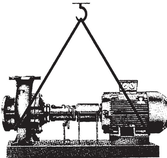
Fig. 2: Transportation of a horizontally mounted pump aggregate
