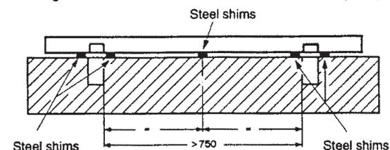
Fig. 3: Alignment with steel shims for horizontal mounting
