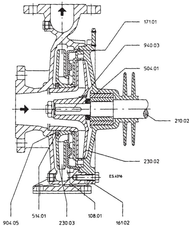
Shaft seal: Uncooled, balanced mechanical seal
