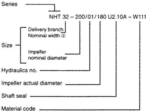
① For the two-stage sizes the number of stages precedes the nominal delivery branch width, separated by a slash, e.g. 2/32-200/...
